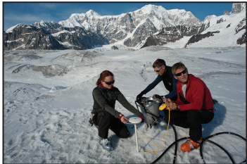
Dr. Michael Loso (red shirt) and collaborators take repeat GPS measurements to calculate glacial ice velocities.
